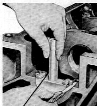
FIG. 33—Seal to Block Installation
