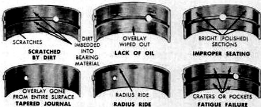
FIG. 21—Typical Bearing Failures
