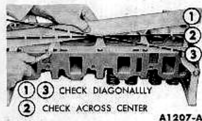
FIG. 5—Cylinder Head Flatness
