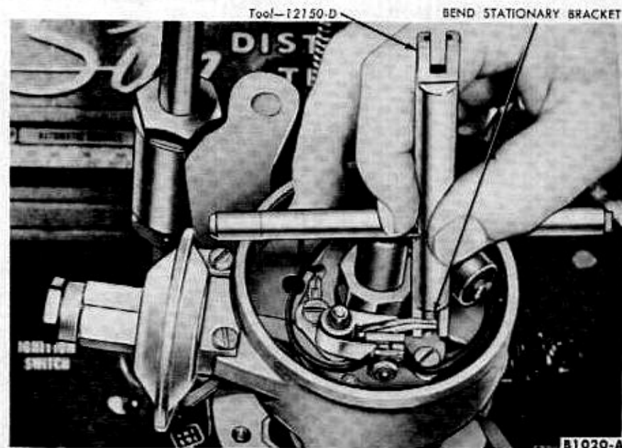
FIG. 14—Aligning Breaker Points
