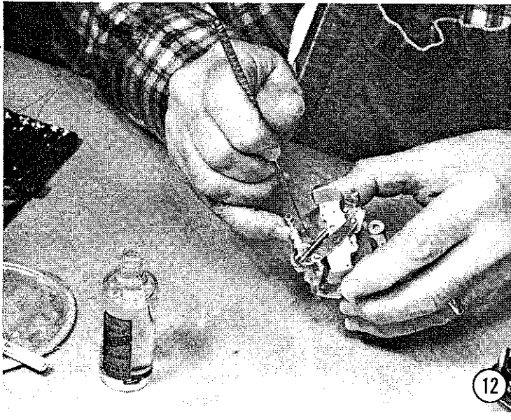
FIGURE 12 — Oiling the Other Side — If you look closely at the balance wheel pivots, you will see that they fit into a couple of hardened steel cones. You will have to put some oil into these. This is pretty easy to do on the side away from the hairspring, but you'll have to be quite careful on the hairspring side — there isn't much clearance. If you get oil on the hairspring, you will have to reclean the clock. Oil on this spring will make two or more turns stick together, which will cause the clock to run fast — about an hour or two a day. Violating the general rule, you will have to put a small amount of oil on the teeth of the escapement wheel. This is the strange looking gear with teeth that look a bit like saw teeth. Put a small amount of oil on every third tooth.
