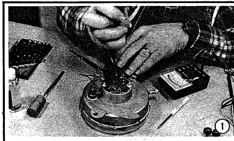
FIGURE 1 shows the removal of the case and terminal nuts. I know that dear old Dad said he'd flatten you if you ever used pliers to remove a nut, but there is little danger of rounding the corners here. Remove the nut that secures the grounding strap to the case. Remember which post you took it from. Also remove any and all screws which fasten the back of the case to the movement.
