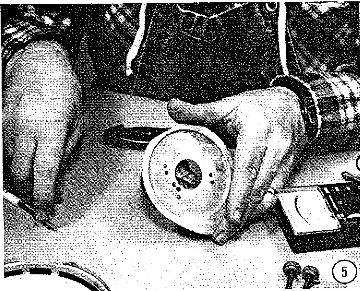
FIGURE 5—Removing the Dial Plate — Figure 5 shows the front of the clock with the dial removed. Notice that the dial plate is held to the movement by three screws and that these screws aren't placed symmetrically. This is to insure that the dial plate can be fastened to the movement in only one orientation. (Ah! The best laid plans, and all that sort of thing.) The dial plate can be reversed, front to back, and still fit. Pay attention or make notes here to avoid some misery later.
