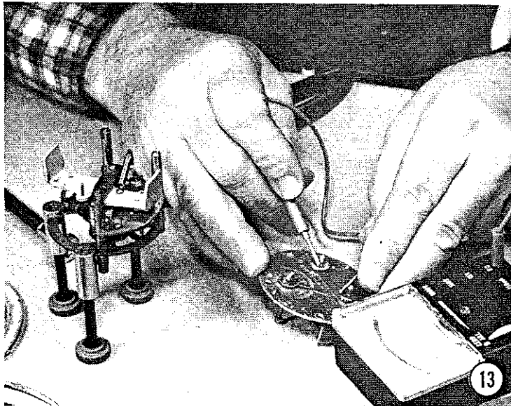
FIGURE 13 — Checking the Resistance — Examine the contact points very closely. If they are pitted, burned, or otherwise corroded, carefully burnish them until they are bright and shiny. Keep your fingers off the contacts to avoid future corrosion from body salts. Snap the contacts closed and measure the circuit resistance, at the wiring terminals, with your ohmmeter. You should get a reading somewhere between 10 to 100 ohms, depending on your clock. If you get a reading in the thousands of ohms, you have an electrical problem. One of your connections is bad. Resoldering all the solder joints with a small soldering iron should take care of this problem. If it doesn't, look for a broken wire (rare). If you can't find one, check directly across the coil; it may be bad (also rare).
